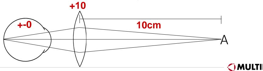
Up to now our Aplanat system was measured/specified in Back vertex power (BVP) and A2 in Equivalent power (EP).
