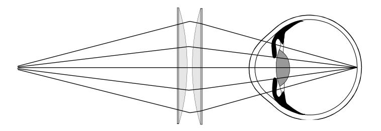
By dividing the power into two lenses and using the plano surface towards eye and object you create an optical system that gives the best optical image AND it is not less sensitive for being off optical centre!
