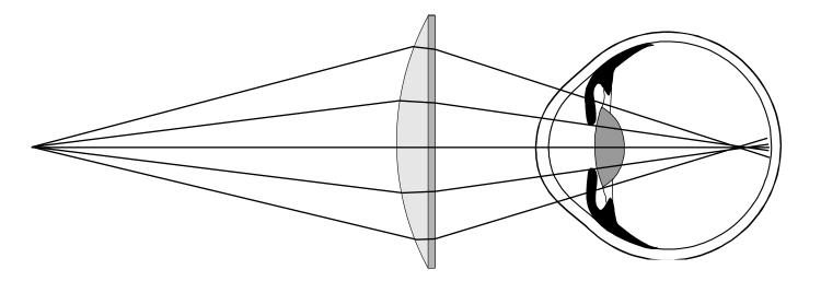
Spherical optics gives some optical errors for the peripheral areas.
