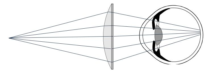
A disadvantage with the aspherical optics is that it's sensitive for being off the optical centre.
