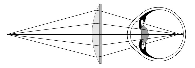
Aspherical optics with lower peripheral curvature corrects this error.
